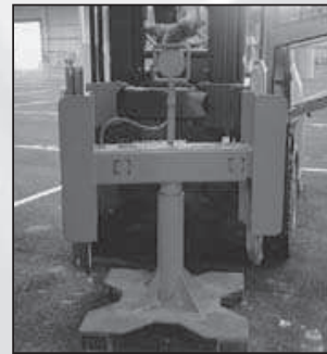
Clamping force testing devices for testing and adjusting the paper roll clamp operation.
