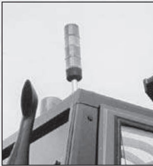
Paper roll clamp pressure selection valves and pressure indication lights for easy clamping force control.
